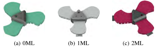
Fig. 3: Three robot configurations: a) baseline aqua SoRo; b) white SoRo with 10 microspines in an array on one limb; c) red SoRo with 20 microspines in two arrays on two limbs.
